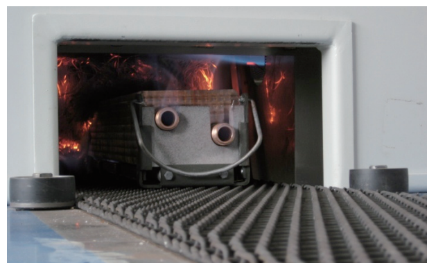
The elements are being sintered by the light soldering method in furnaces.
